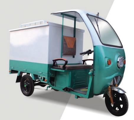
Climbing ability: 15-20 Degree Minimum turning radius: 5M Compartments Size (mm): 1300\*950\*1000 Outline Size (mm):2856\*1000\*1730 Steel thickness (mm): 1.2 Brake type: drum brakes
