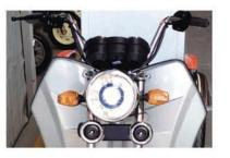
Power: 500W Voltage: 48V Battery Capacity: 45Ah Max Speed (km/h): 35-40 km/h Once timing Mileage (Km): 40km Climbing Ability: 0-25 Degree Minimum Turning radius: 5M Outline Size (mm): 2550\*850\*1230
